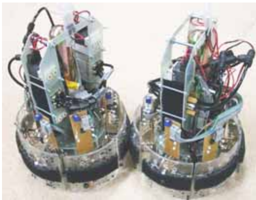
Fig.4: A photo of the prototype of Slimebot (two physically-connected modules are shown).
