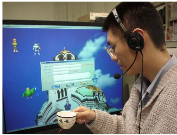
(b) Conversation with CAs. A cup inquires a question to a user. The user replies to him by using a microphone connecting to the server. Answers from the user is stored in gossip database in the server, and utilized as gossip data.
