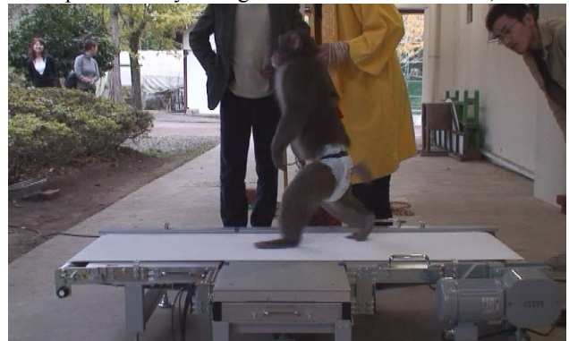
Fig 3. Synchronous measurement of locomotor kinematics and kinetics using a new treadmill in which a force plate could be embedded.
