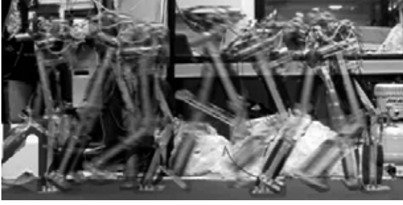
Fig. 6. Running experiment: the flight time and speed were 0.12[s] and 1.13[m/s], respectively. Air pressure was 0.6[MPa]. It could run 5 steps at most.
