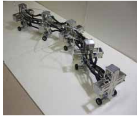
Fig. 11. A Snake robot prototype driven by pneumatic actuators
