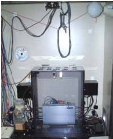
Figure 1 Apparatus of behavioral tasks. In the operant box located in the center, rats are trained to perform behavioral tasks. The interface box to control the operant box and other apparatuses is set behind the box. The loud speaker and cables with head-amplifiers are attached near the ceiling. All are in the sound-proofed shielded box .
